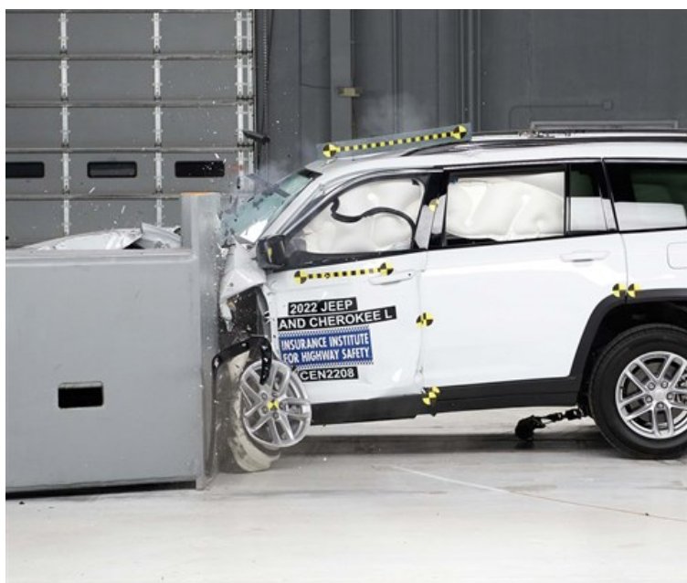
Action shot taken during the driver-side small overlap frontal crash test.
