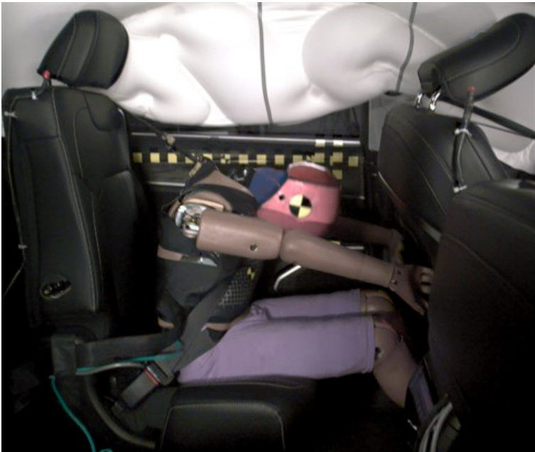
The rear passenger dummy's head approached the front seatback, which increases the risk of head injuries.
