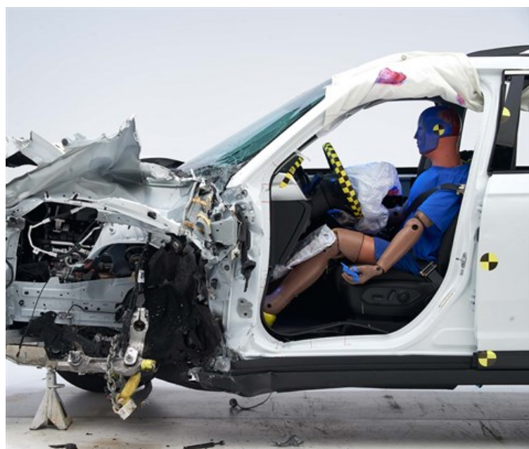
The dummy's position in relation to the door frame, steering wheel, and instrument panel after the crash test
