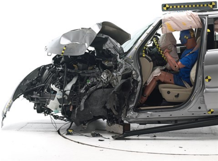
The dummy's position in relation to the door frame, steering wheel, and instrument panel after the crash test indicates that the driver's survival space was not maintained well.
