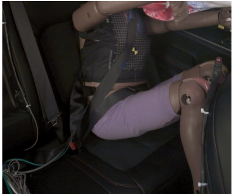
The rear passenger dummy's lap belt remained in the ideal position on the pelvis.
