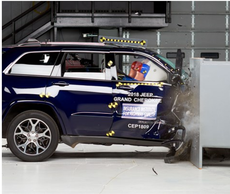
Action shot taken during the passenger-side small overlap frontal crash test.
