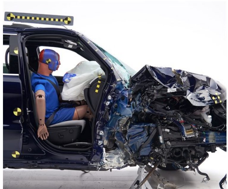
The dummy's position in relation to the door frame and dashboard after the crash test indicates that the passenger's survival space was not maintained well.
