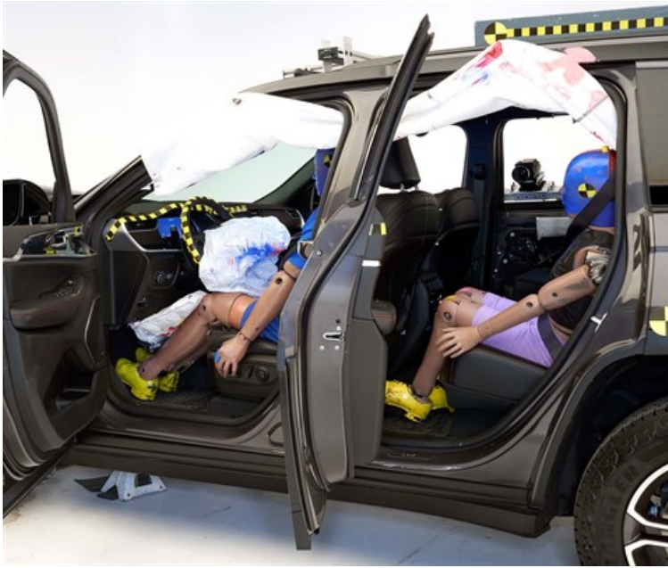
View of the vehicle after the crash showing the airbags and damage to the occupant compartment.
