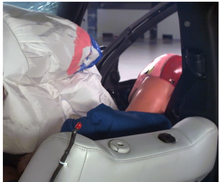
The passenger door opened during the crash test, and the dummy's head moved outside the vehicle during rebound.
