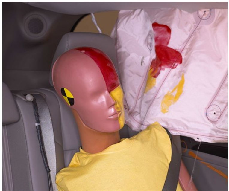
Smeared greasepaint shows where the rear passenger dummy's head was protected by the side airbag.
