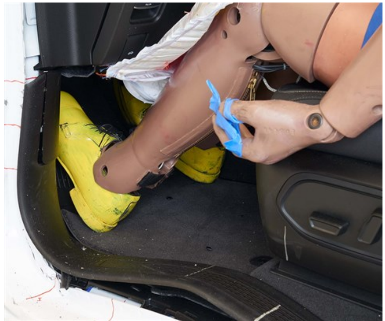
The driver's space was maintained well, and risk of injuries to the dummy's legs and feet was low.
