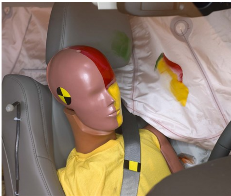
Smeared greasepaint shows where the driver dummy's head was protected from being hit by hard structures by the side curtain airbag.
