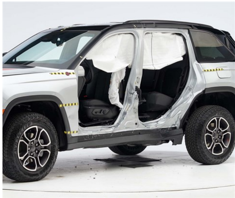
View of the vehicle after the crash with doors removed, showing the side airbags and damage to the occupant
