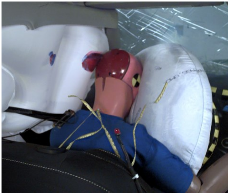
The frontal and side curtain airbags worked well together to keep the head from coming close to any stiff structure or outside objects that could cause injury.
