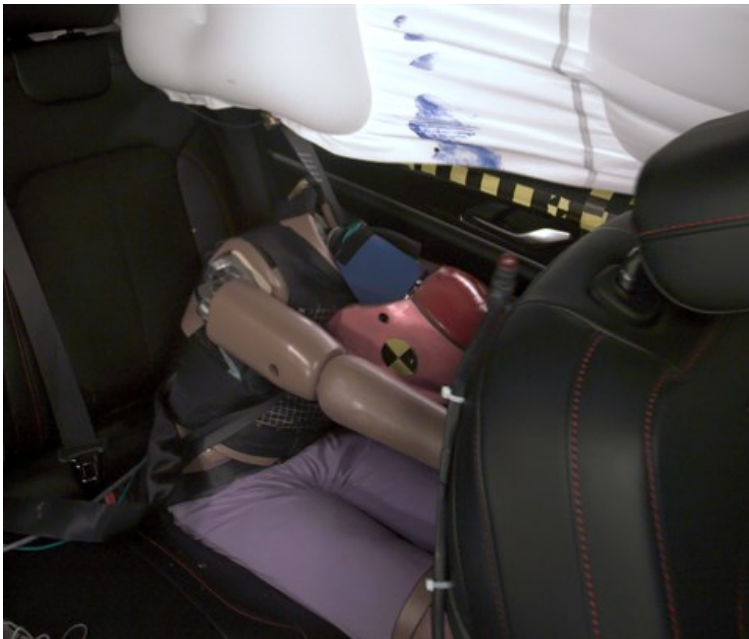
Rear passenger dummy injury values indicate a likely risk of injury to the head or neck and chest. During the crash, the shoulder belt remained in an ideal position on the dummy's chest.
