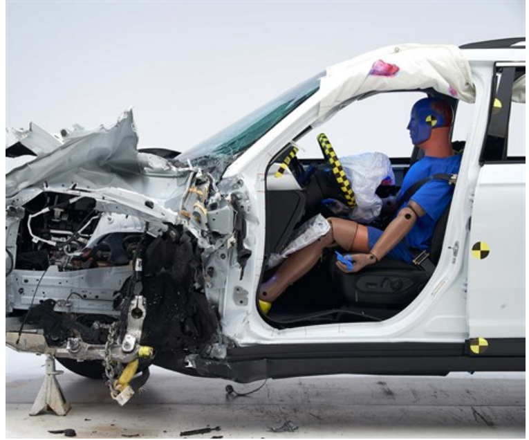
The dummy's position in relation to the door frame, steering wheel, and instrument panel after the crash test indicates that the driver's survival space was maintained very well.
