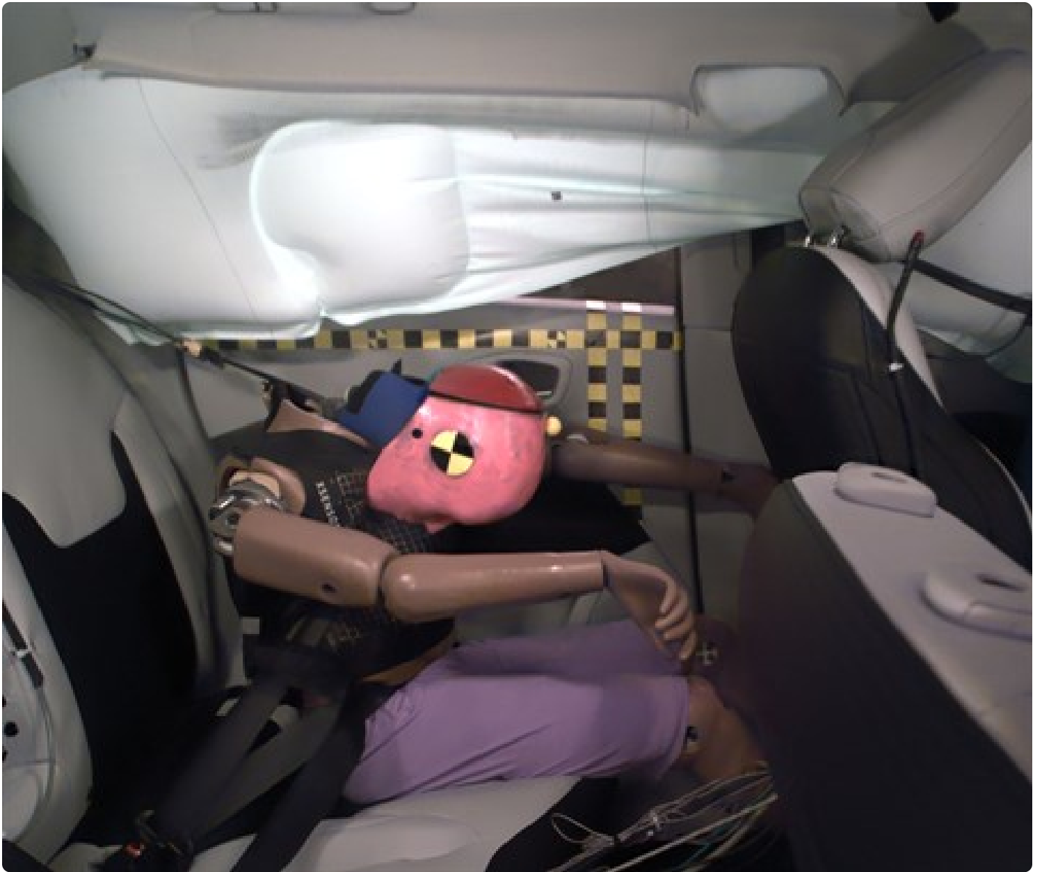
The rear passenger dummy's head remained a safe distance from the front seatback.
