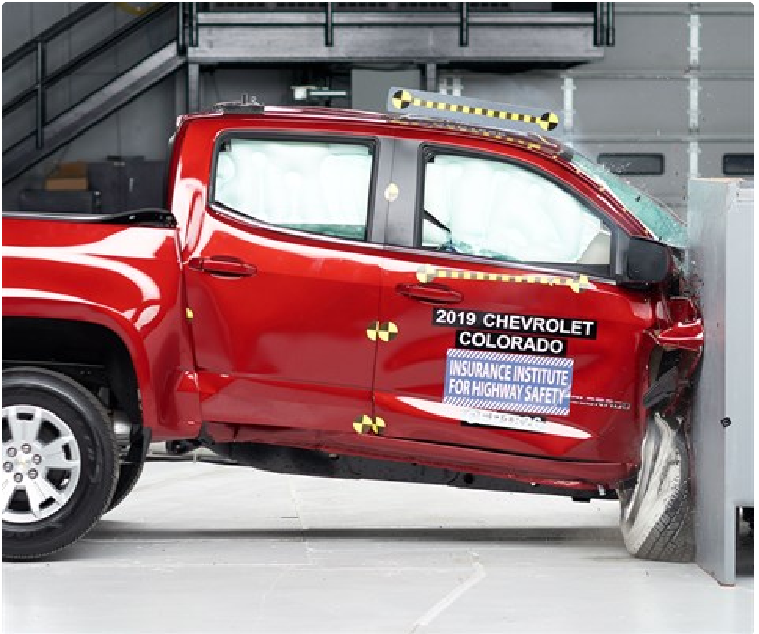
Action shot taken during the passenger-side small overlap frontal crash test.
