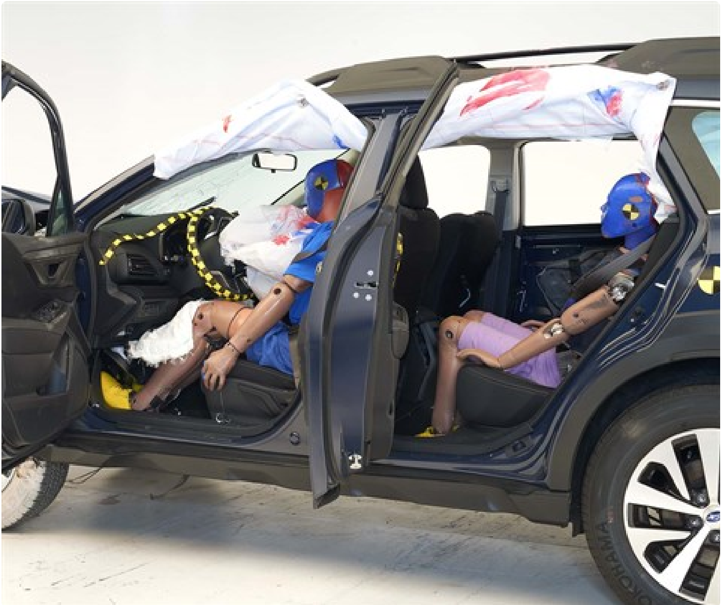
View of the vehicle after the crash showing the airbags and damage to the occupant compartment.
