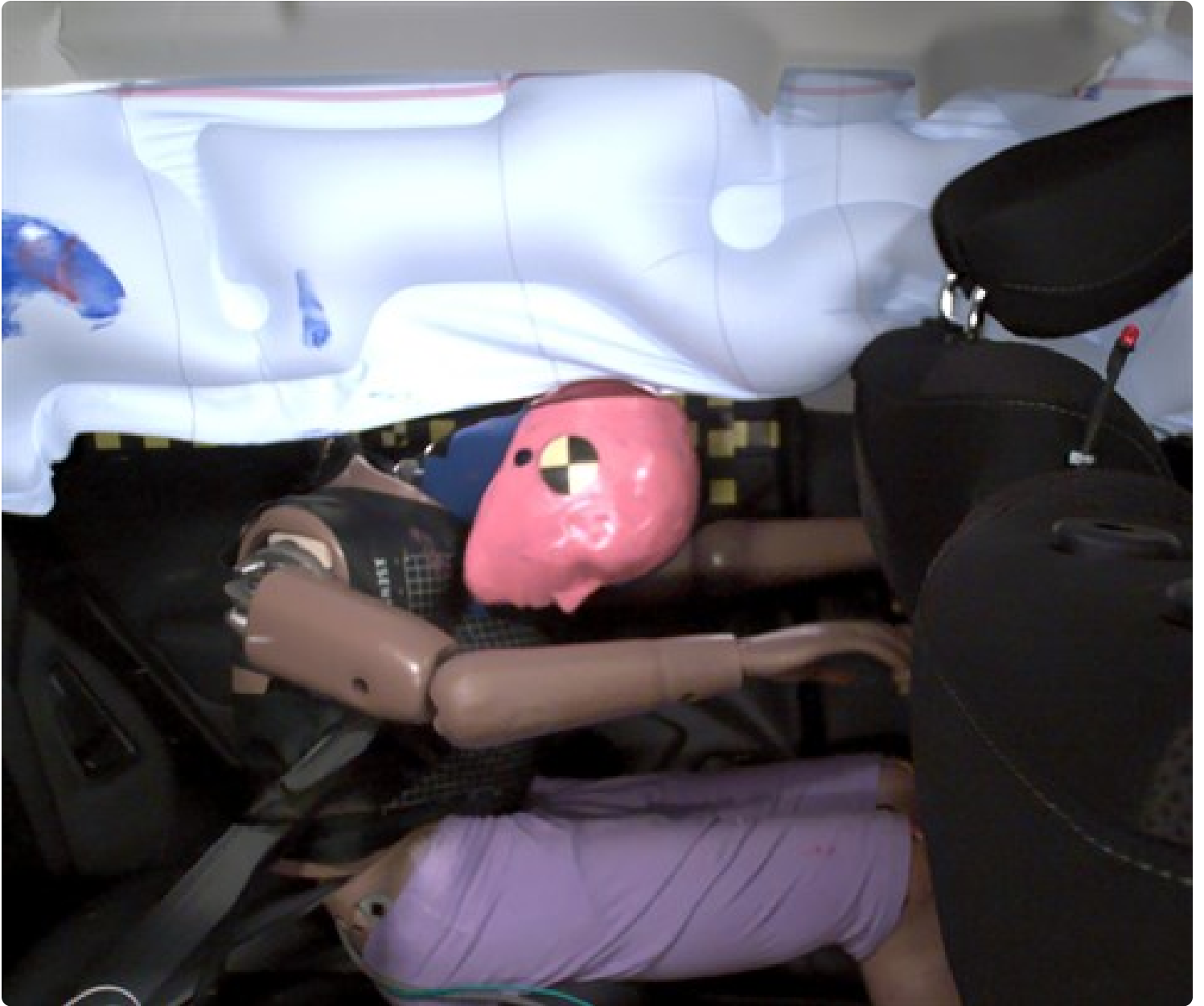
The rear passenger dummy's head approached the front seatback, which increases the risk of head injuries.
