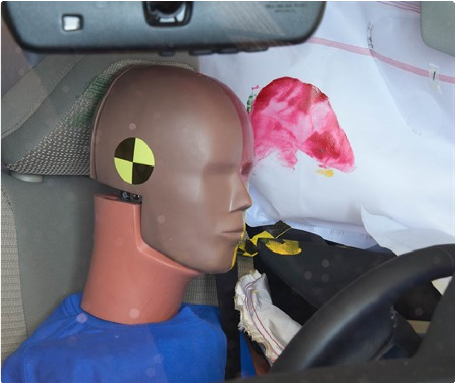
Smearred greasepaint shows where the driver dummy's head was protected from being hit by hard structures by the side airbags.
