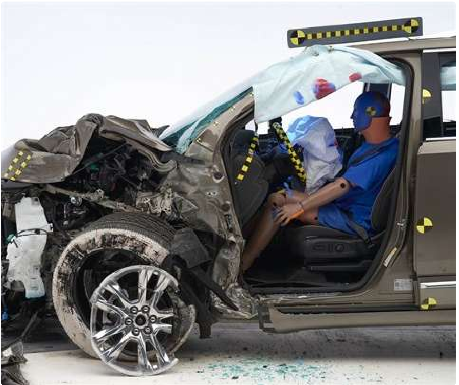
The dummy's position in relation to the door frame, steering wheel, and instrument panel after the crash test indicates that the driver's survival space was maintained well.
