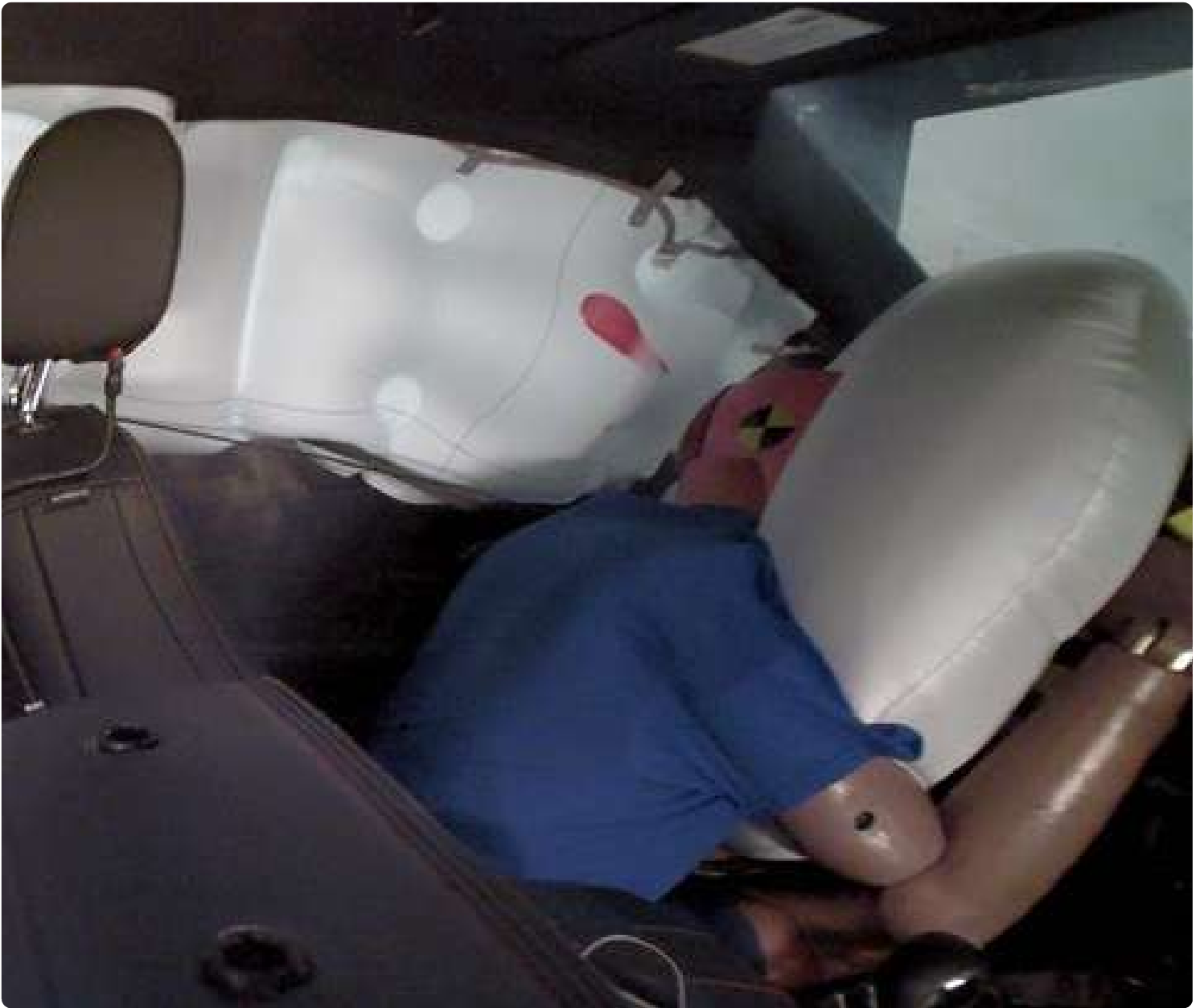
During the crash, the driver dummy's head hit the steering wheel hard through the airbag.
