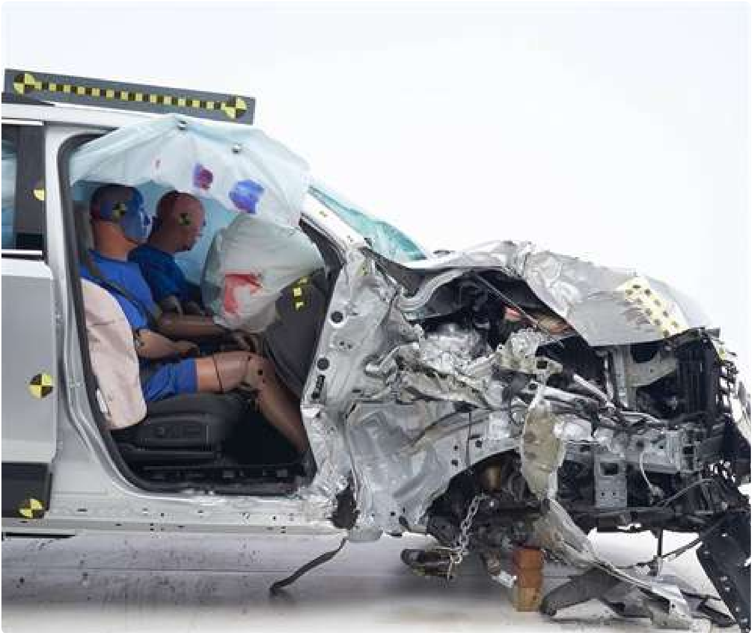
The dummy's position in relation to the door frame and dashboard after the crash test indicates that the passenger's survival space was maintained reasonably well.
