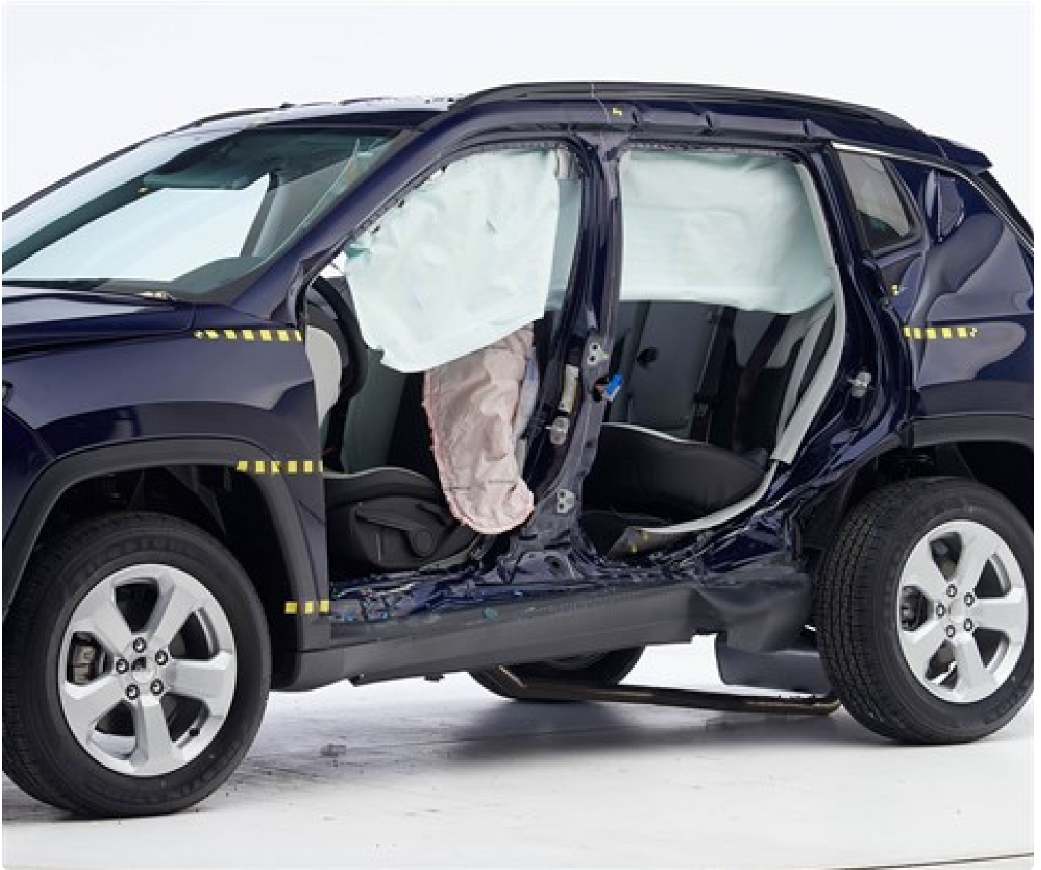
View of the vehicle after the crash with doors removed, showing the side airbags and damage to the occupant compartment.
