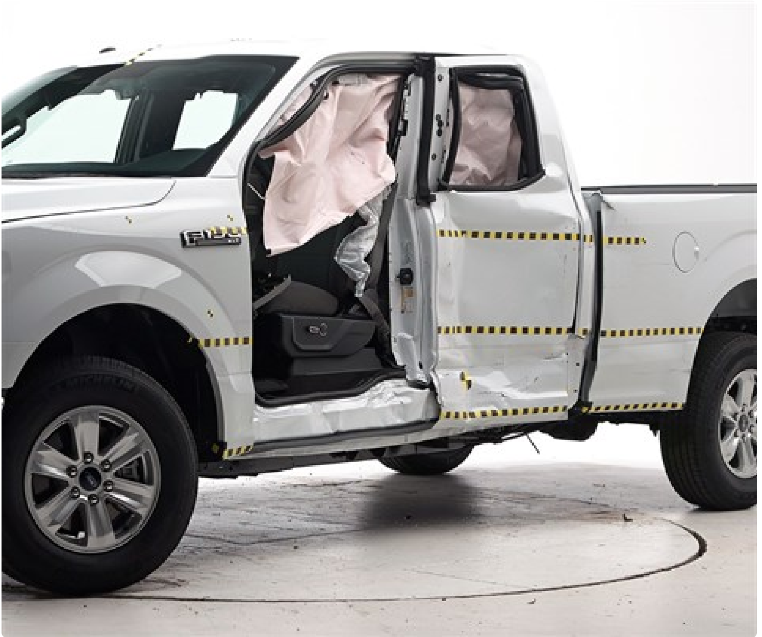
View of the vehicle after the crash with the front door removed, showing the side airbags and damage to the occupant compartment.
