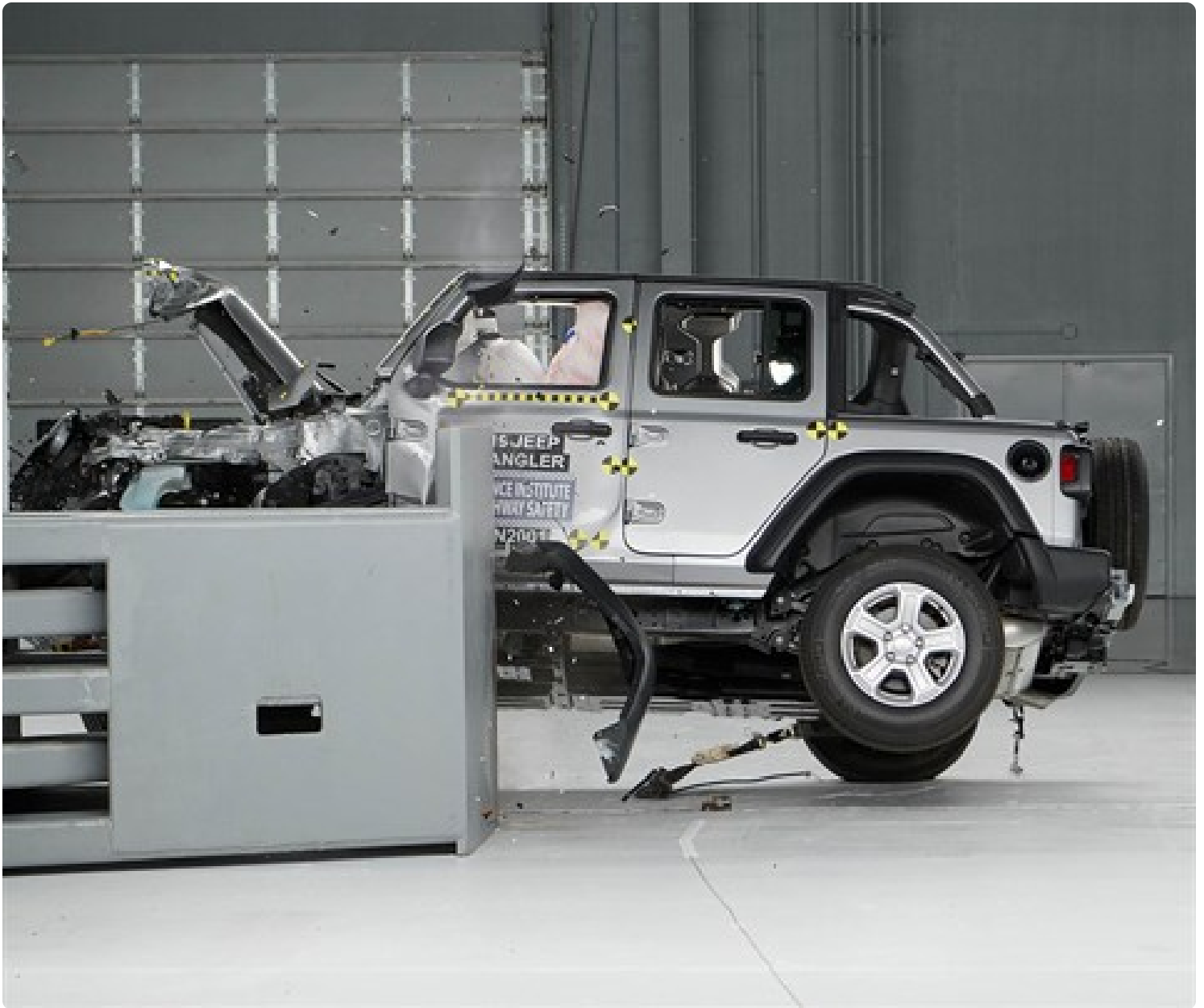
Action shot taken during the second of two Institute-conducted driver-side small overlap frontal crash tests just before the vehicle tipped on its side.
