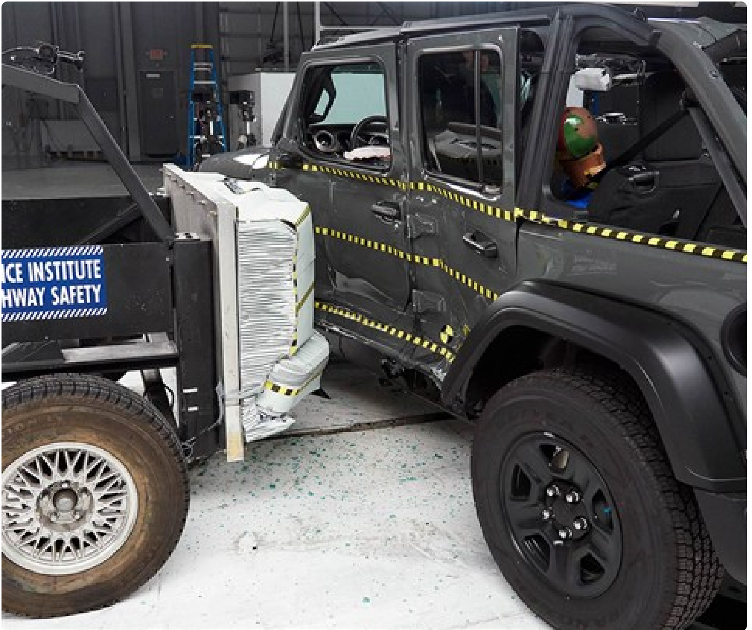
View of the vehicle and barrier just after the crash test.
