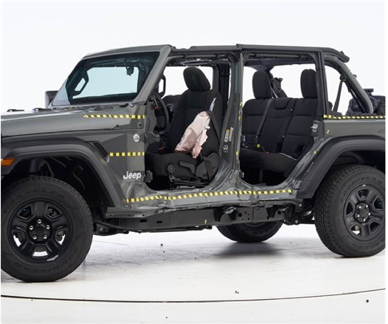
View of the vehicle after the crash with doors removed, showing the driver side airbag and damage to the occupant compartment.
