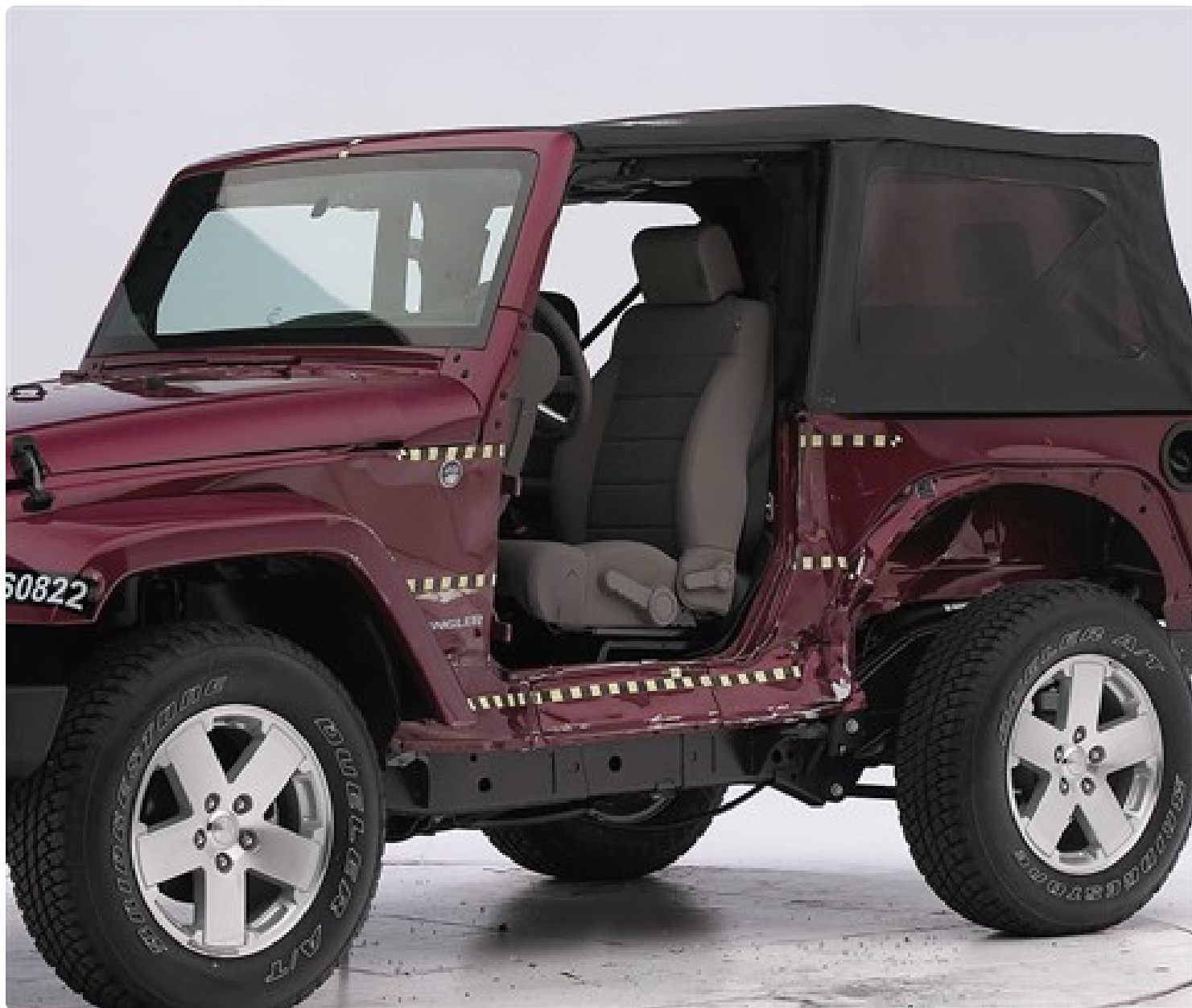
View of the vehicle after the crash with door removed, showing damage to the occupant compartment.
