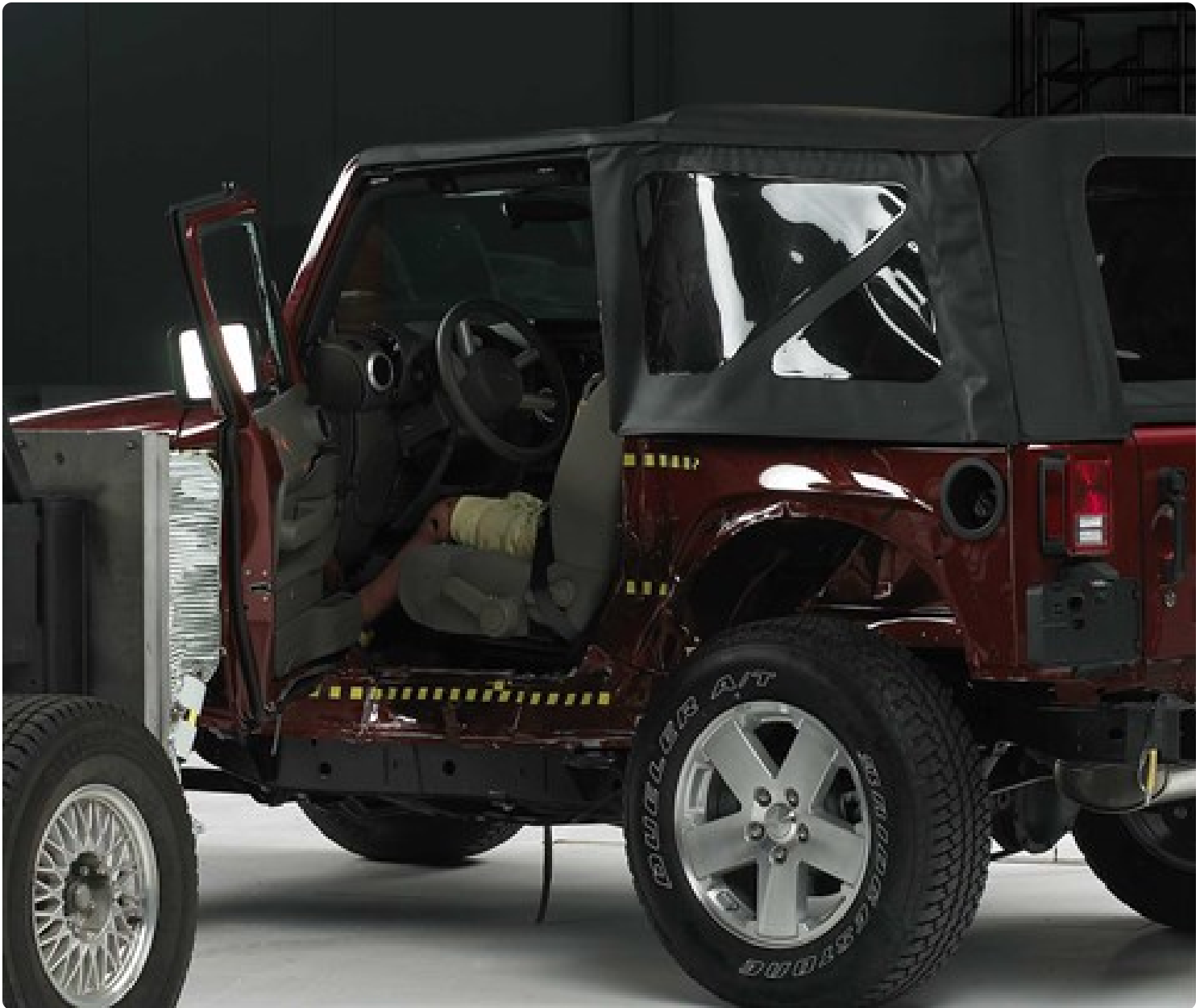
View of the vehicle and barrier just after the crash test, showing the open driver door.
