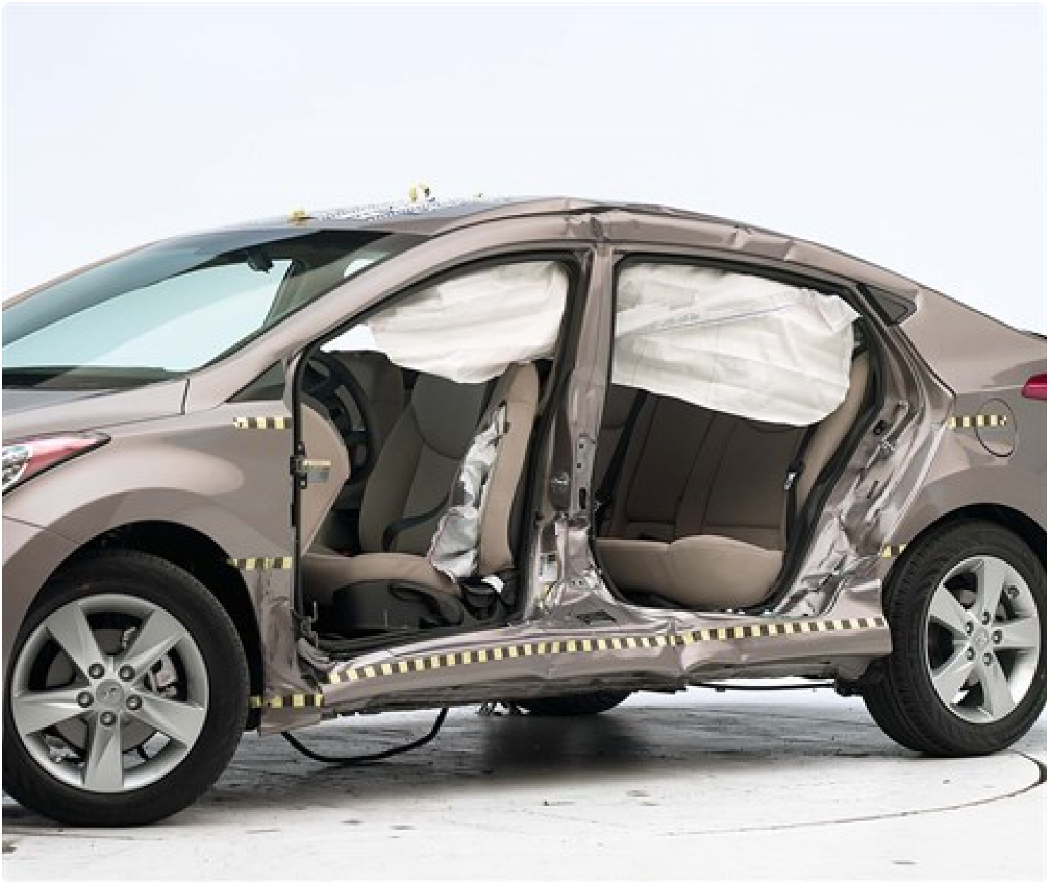
View of the vehicle after the crash with doors removed, showing the side airbags and damage to the occupant compartment (Institute test car shown).
