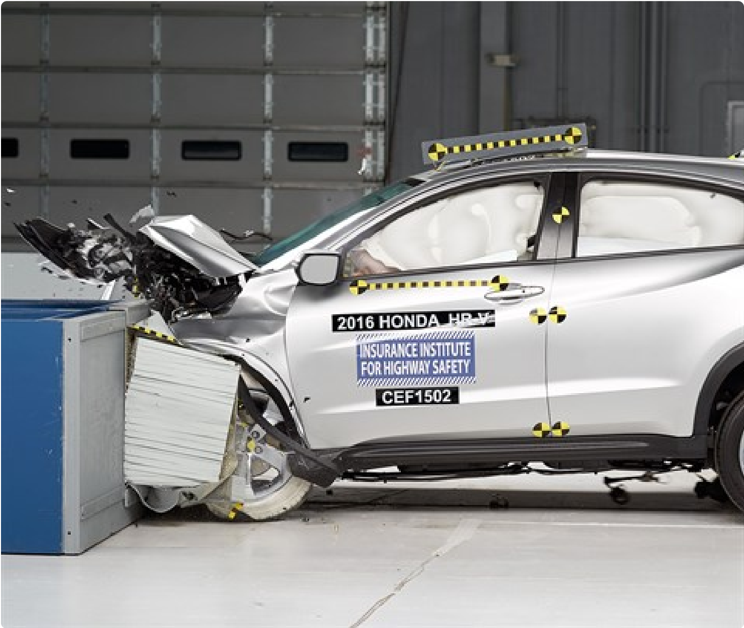
Action shot taken during the moderate overlap frontal crash test.
