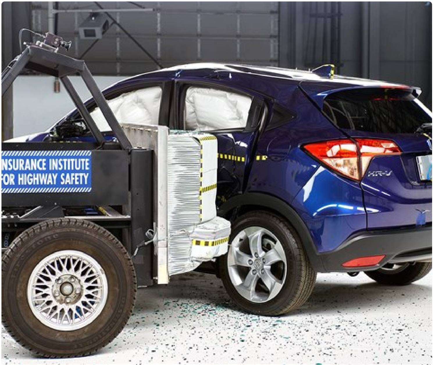
View of the 2016 Honda HR-V and barrier just after the crash test.
