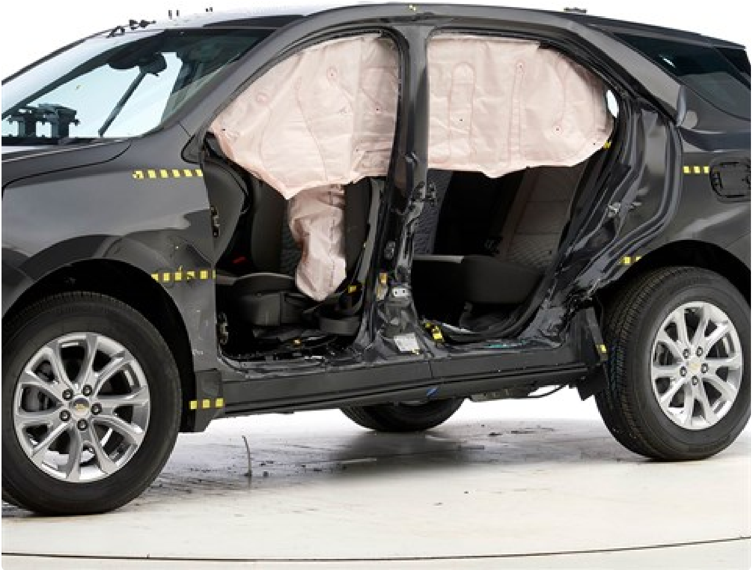
View of the vehicle after the crash with doors removed, showing the side airbags and damage to the occupant compartment.
