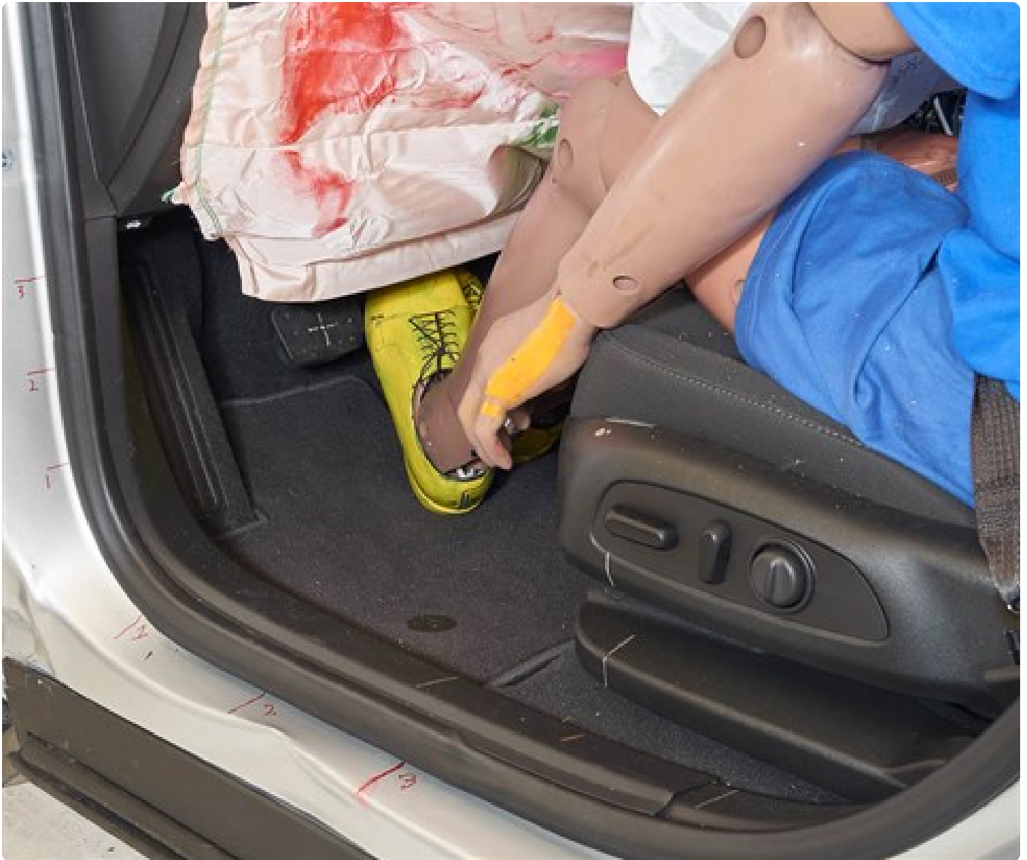
The driver's space was maintained well, and risk of injuries to the dummy's legs and feet was very low.
