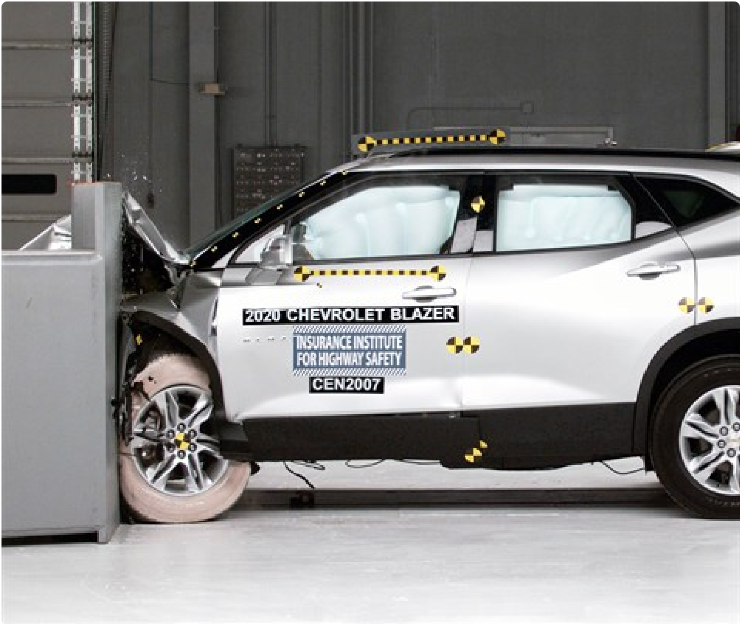
Action shot taken during the driver-side small overlap frontal crash test.
