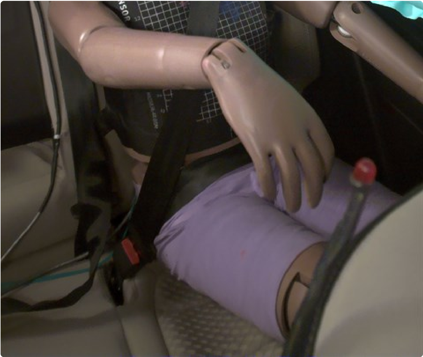
The rear passenger dummy's lap belt remained in the ideal position on the pelvis.
