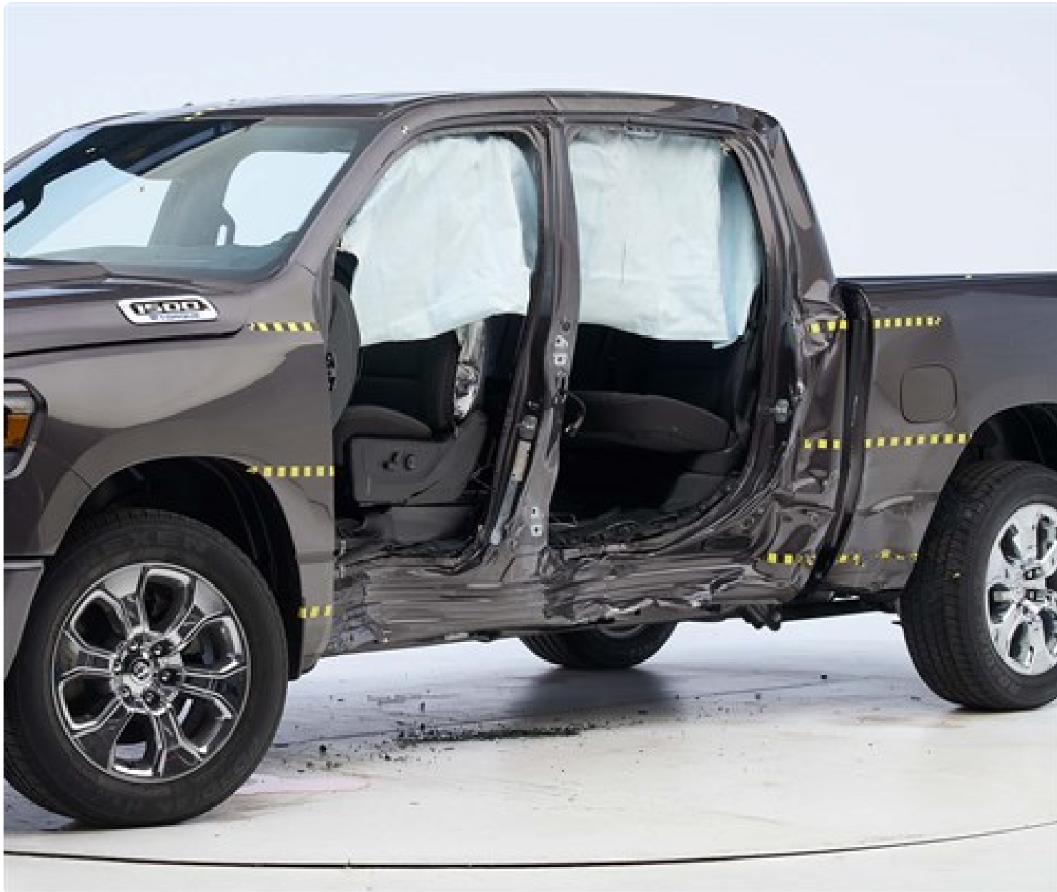
View of the vehicle after the crash with doors removed, showing the side airbags and damage to the occupant compartment.
