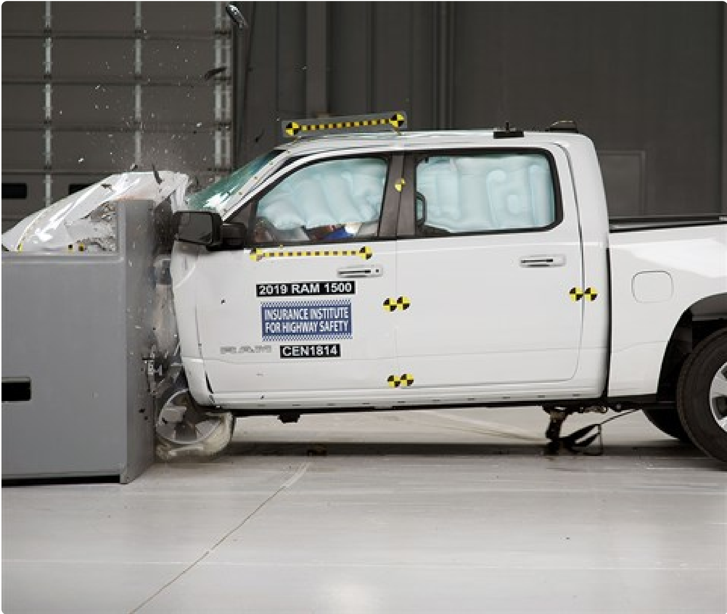
Action shot taken during the second of two driver-side small overlap frontal crash tests.
