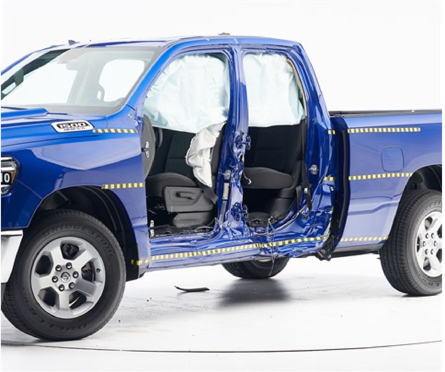
View of the vehicle after the crash with doors removed, showing the side airbags and damage to the occupant compartment (Institute test vehicle shown).
