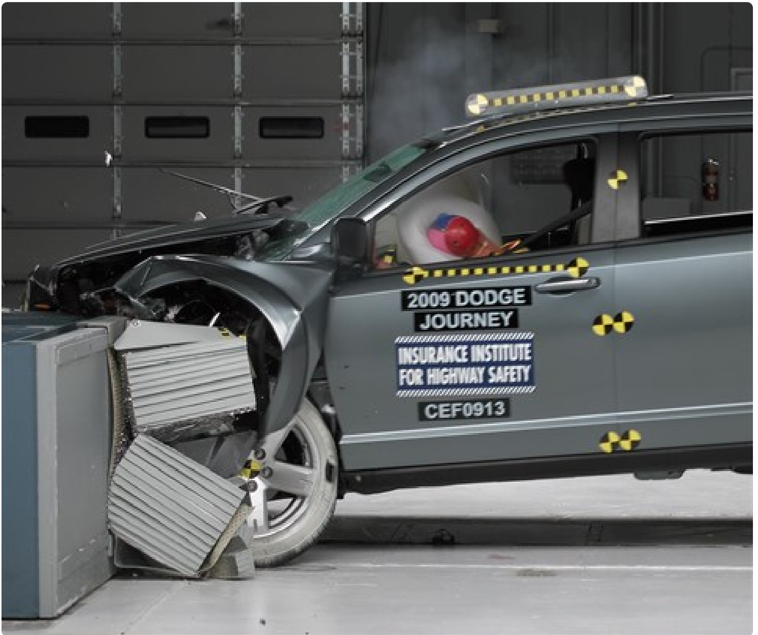
Action shot taken during the frontal offset crash test.
